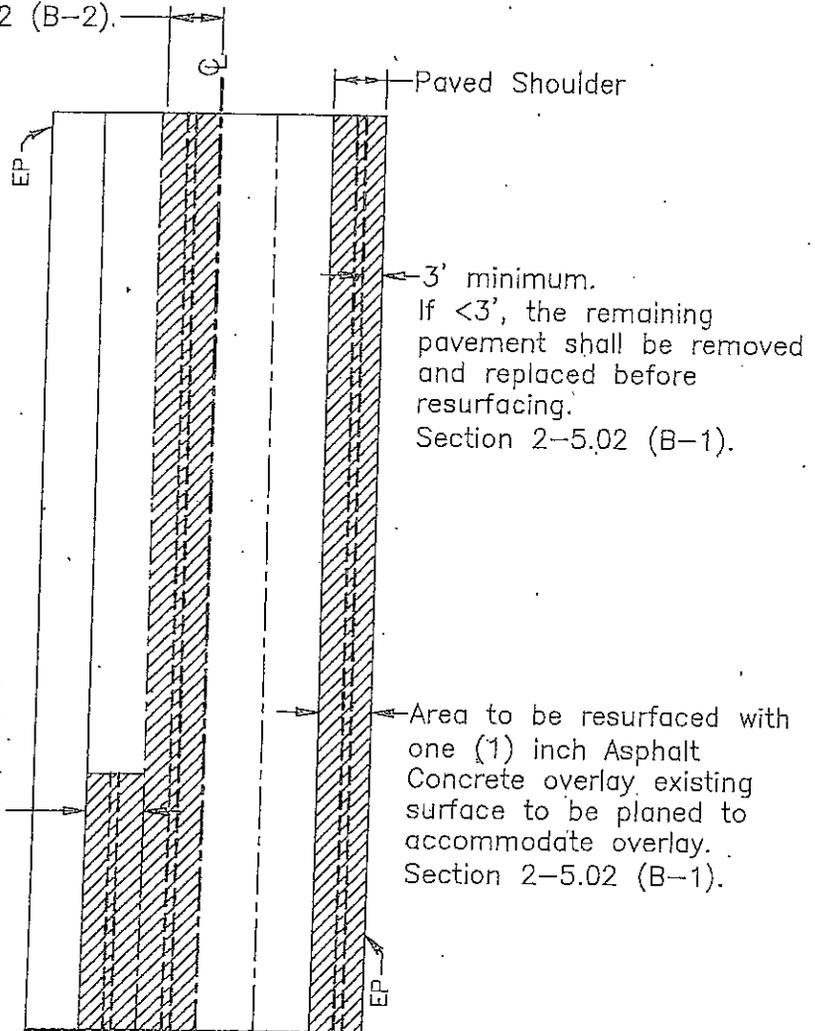
Area to be resurfaced with one (1) inch Asphalt Concrete overlay existing surface to be planed to accommodate overlay. Section 2-5.02 (B-2)
