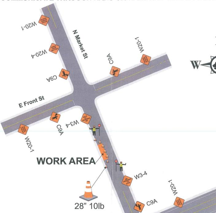
SIGN SPACING TAPER TANGENT SPEED **TAPER** 25 125' 100' 25 180' 30 60 245' 35 70 250" 320' 40 80 45 90 350' 50 600' 100
