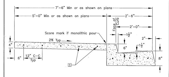
VERTICAL CURB, GUTTER AND SIDEWALK
