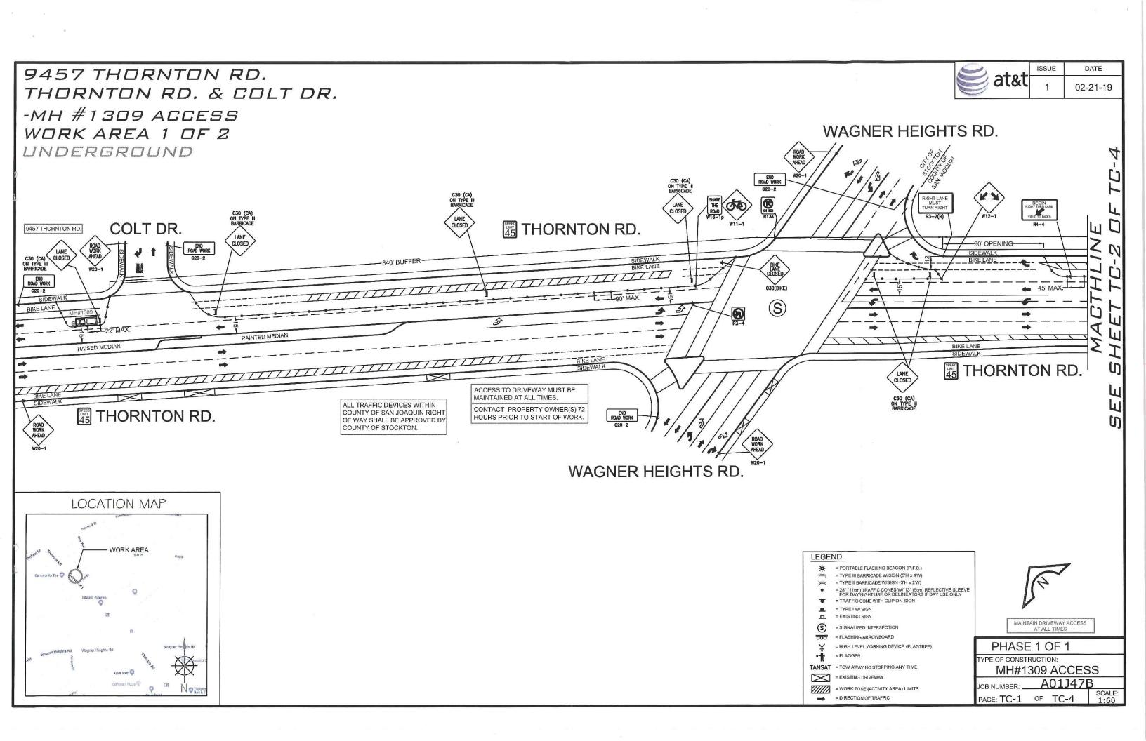
9457 THORNTON RD. ISSUE DATE at&t THORNTON RD. & COLT DR. 02-21-19 -MH #1309 ACCESS WORK AREA 1 OF 2 UNDERGROUND ACCESS TO DRIVEWAY MUST BE ALL TRAFFIC DEVICES WITHIN MAINTAINED AT ALL TIMES. COUNTY OF SAN JOAQUIN RIGHT OF WAY SHALL BE APPROVED BY CONTACT PROPERTY OWNER(S) 72 COUNTY OF STOCKTON. HOURS PRIOR TO START OF WORK. THORNTON RD. CONNIE AVE. FLASHING ጭው RROW BOARD -540' MERGE TAPER 180' BIKE TAPER CITY OF STOCKTON
