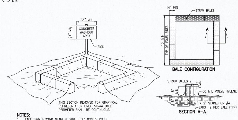
FACE SIGN TOWARD NEAREST STREET OR ACCESS POINT. CONCRETE WASHOUT SHALL BE LOCATED BEHIND THE CURB AND 50 FEET MINIMUM FROM DRAINAGE INLETS OR WATERCOURSES. CONTRACTOR SHALL CONDUCT ALL CONCRETE WASHOUT OFF-SITE. WASH OUT SHALL BE CONSTRUCTED PER CASQA BMP MEASURES OR EQUIVALENT.
