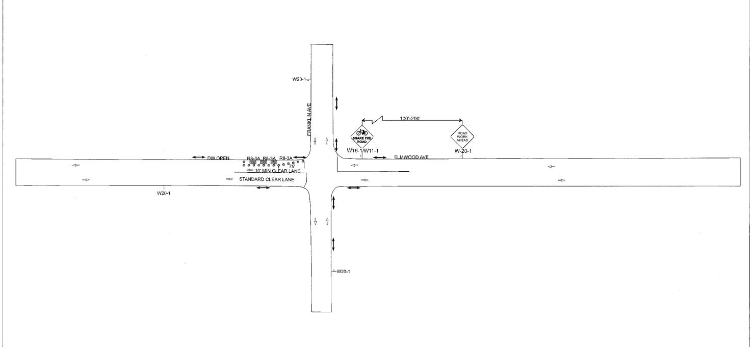
POSTED SPEED: 25 MPH 1/3 SHOULDER TAPER 75' CONE SPACING: 25' SIGN SPACING: 100-200' BUFFER ZONE: OPTIONAL 25 MPH 10' OFFSET = 11' OFFSET = 12' OFFSET = CLICENSE # 975518 (916) 452-4855
