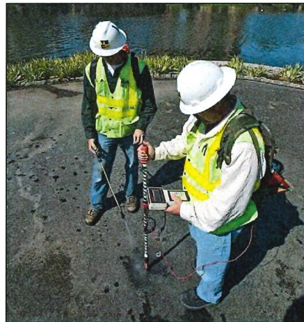
DAMPEN SOIL TO IMPROVE DEVICE CONNECTION TO SOILS.
