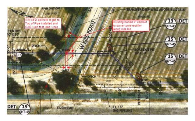
The existing conduit in the ground along the shoulder was installed under a previous corrosion workstream project (C-719). We will be utilizing the conduit to run new wires from the new pipeline (bellhole excavation) back to the adjacent power pole. No planned excavation aside from the bellhole to access the newly installed pipeline and CAD weld new wires to the pipeline. Backfill and restoration per County Improvement Standards R-29, R-36, & R-37
